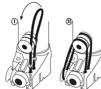
**B** Rope Threading for rotated tack pulleys (90° position) e.g. Severne, Gun Sails, Naish
