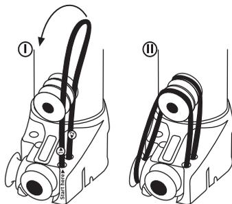
**B** Rope Threading for rotated tack pulleys (90° position) e.g. Severne, Gun Sails, Naish
