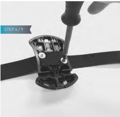
Now turn the base upside down, take a Philips-head screw-driver and fix the webbing to the base with 2 screws and washers.
